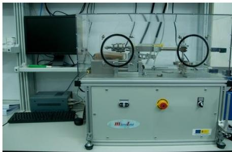
Figura 31: Tribómetro "Pin on Disk" (Microtest)
